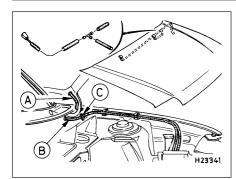
19.16 Routing of washer hoses in the engine compartment
